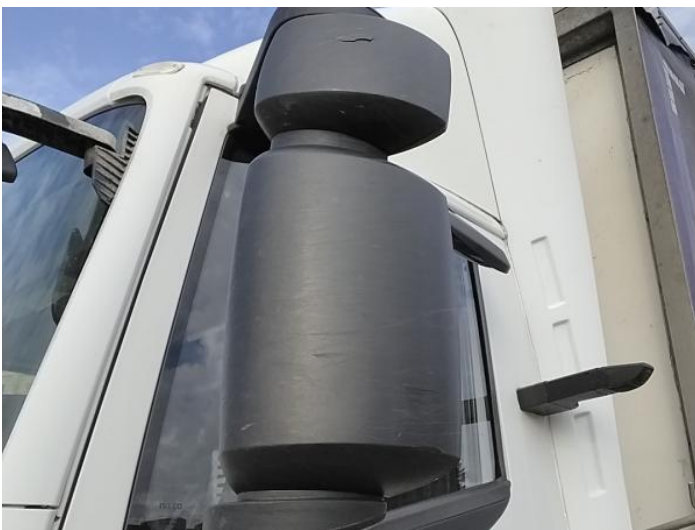
7: Door Mirror Assy nsf Broken Replace
