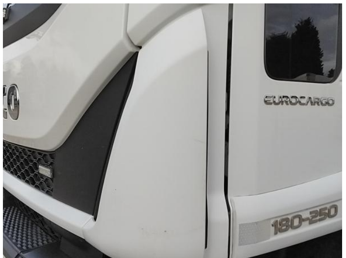
8: Wing nsf Scratched UpTo 25mm Not Thru Paint
