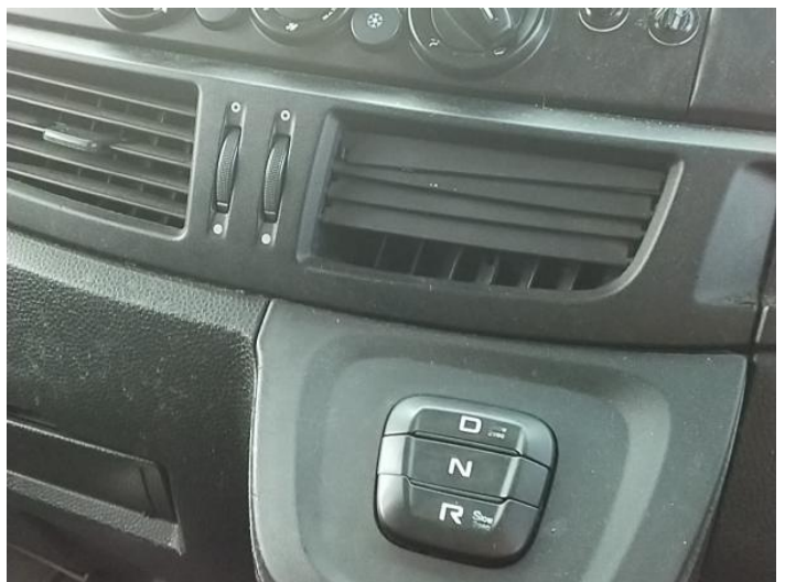
14: Air Vents osf Damaged Replace
