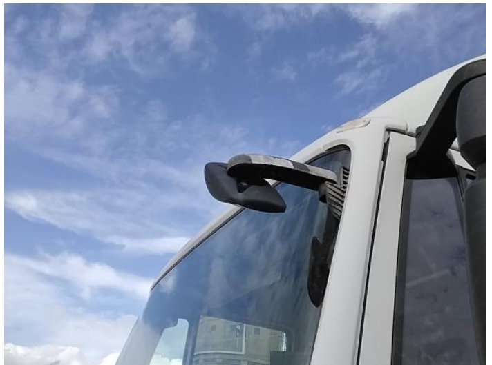
6: Door Mirror Assy nsf Broken Replace
